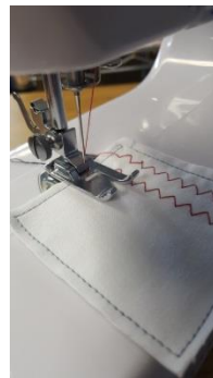
Raised Needle when turning
